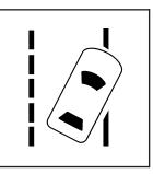
When the vehicle is started, the LDW symbol, located in the instrument panel cluster, will briefly come on to indicate that the light is operational.
